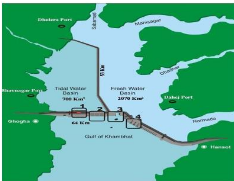
Figure 2.4 The first alternative with a tidal basin
